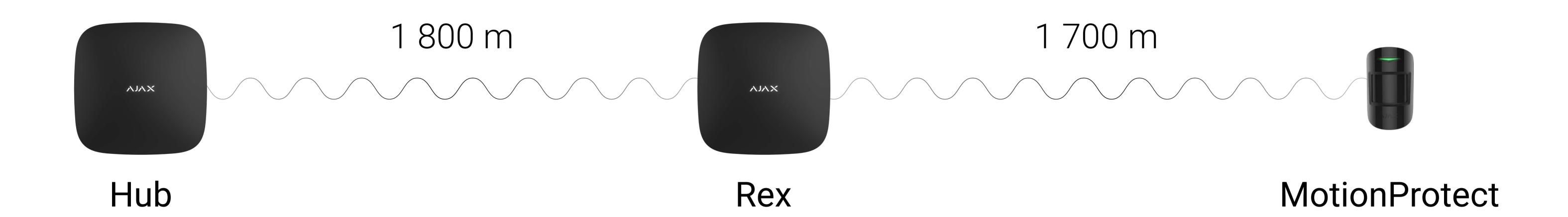
The maximum range of radio communication with connected devices is 1700 meters without obstacles. Up to 5 range extenders can be connected to the Ajax security system. It allows using Ajax products for largescale facilities protection. Regardless of the number of devices connected to the ReX, alarms are delivered in 0.3 seconds.
